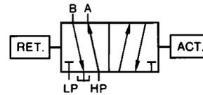
**3 POSITION 5/3** Diagrams below show center position only. Offset positions are same as shown above for 2-position types. To indicate particular center pattern, substitute number shown within corresponding diagram for fourth digit of product number.
