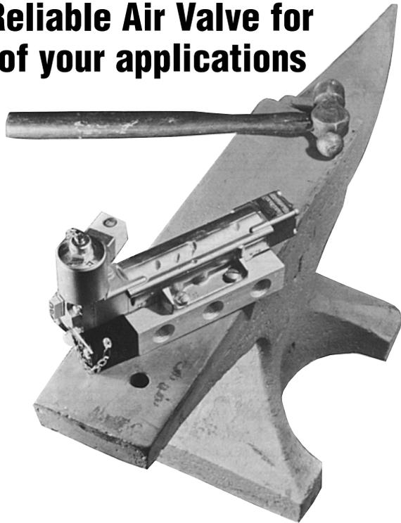
All of Versa's Series V & T valves are rugged in design and construction. All provide thick-walled forged-brass bodies and rod brass internal parts. The RUGGD<sup>®</sup> valves featured here are solenoid operated versions of the standard Series V valve to which several options have been added and offered as standard for the RUGGD<sup>®</sup> line of valves.
