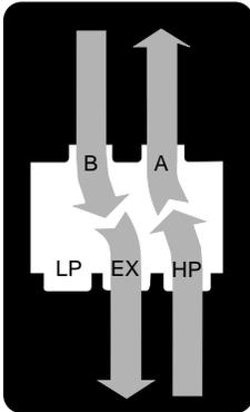
HP inlet open to cylinder port A;
