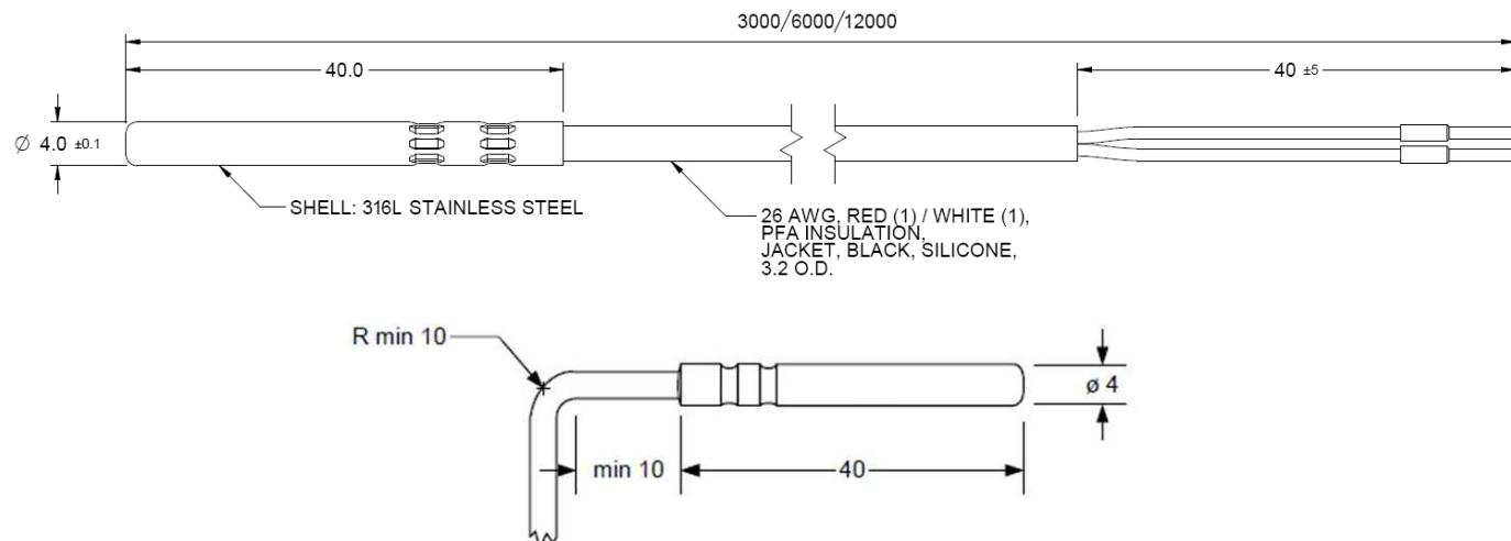
\*Cable should not be bent at distance less than 10mm from the end of probe's housing
