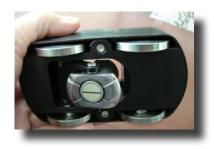
The **EZ Scan 4** is a small, single axis linear B-Scan encoder, for use with the T-Gage V DLC, with magnetic wheels and a couplant delivery system. Ideal applications include storage tank bottom and side walls, flat plates and pipes with a 10 cm (4") or greater outside diameter. The scanner comes as standard with a 5Mhz dual transducer spring loaded in two directions, other transducers are also available.
