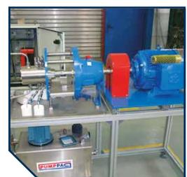
EDI Test rig for Pump packing
