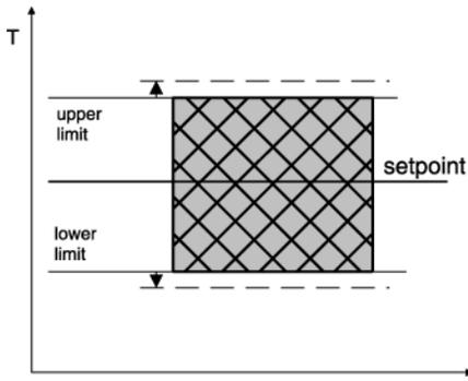
**Fig. 4:** Range alarm, alarm contact normal
