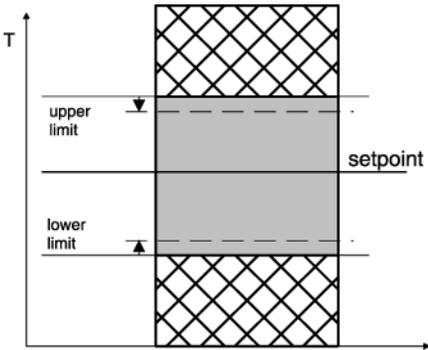
**Fig. 5:** Boundary alarm, alarm contact invers
