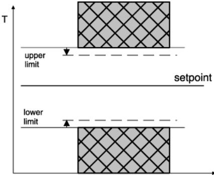
**Fig. 3:** Boundary alarm, alarm contact normal
