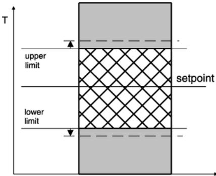
**Fig. 6:** Range alarm, alarm contact invers
